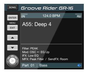
Display area is located at the left of the Top Panel. It has a Display, four buttons (**ENTER**, **EXIT**, **UP**, **DOWN**) to navigate through the menus, a **SONG** button, and a Value Jog knob, which can be used to change menu values, selected with a cursor.
