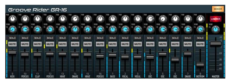
On the Mixer Page, you can see all 16 Parts at one time as mixer channels. In this view, you have an instant access to every Part's Level fader, Pan knob, Send FX knob, as well as Part's Mute and Solo buttons. This helps to instantly adjust the mix of the Pattern by controlling all the Parts at one time on one page. At the right, you can see a Master Volume fader, which has its unique value, stored for each Pattern.
